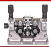
Expert model is fitted with 'Mechafin' Swiss made 4 roll wire drive for precision feeding of filler wires at speeds from 0.2M/min-18M/min A huge range of roller sizes & profiles are available for this model.
